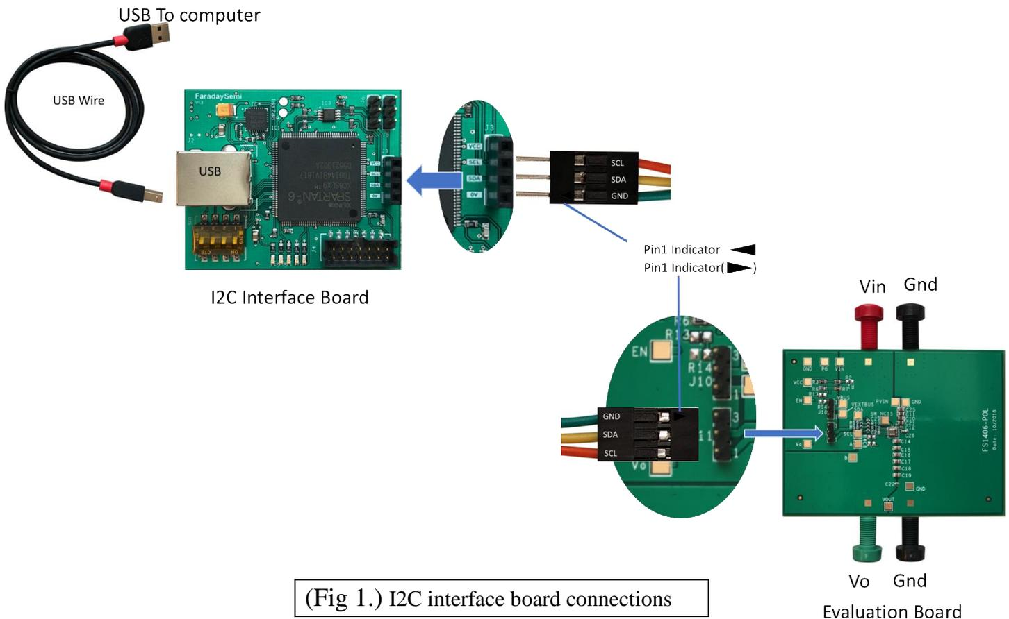
(Fig 1.) I2C interface board connections
