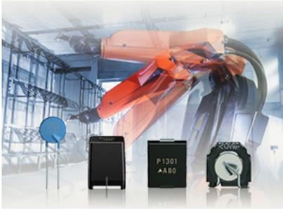
One of the properties of PTC thermistors is that when an excessively large current flows, they generate heat by themselves and become highly resistive. With this property, they are used as overcurrent protection devices.
