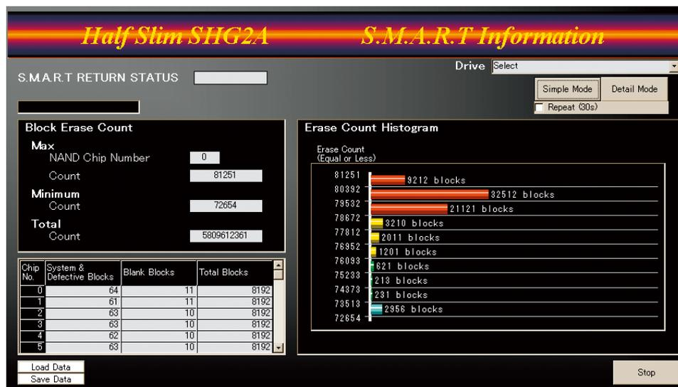
Monitors number of program (erase) counts of TDK CompactFlash cards or SSDs (SMART ON compatible models) and calculates estimated service life in real time.
