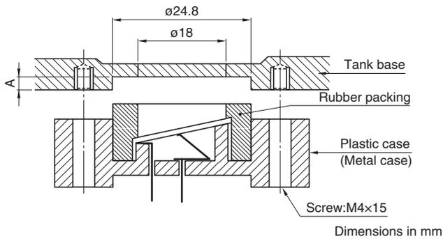
The transducer can break off if the A dimension depth is shallow. TDK recommends a 2mm A-dimension depth and a screw tightening torque of  $0.39\text{N} \cdot \text{m}$ .
