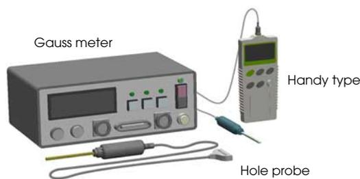
The gauss meter and hole probe are used together to measure magnetic flux density. The measurement accuracy is achieved using probe stands and such, which reduce the unevenness of predetermined measurement conditions (such as the degree of close contact, interval, or parallelization between the hole probe and measured objects).
