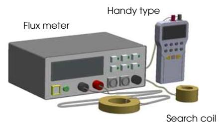
The flux meter with attached search coils is used to measure the amount of magnetic flux of each product. Measurement values can still differ because of inconsistent speeds of magnet movements and separation distances from the search coils.
