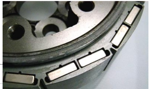
High performance neodymium magnet for IPM motor
