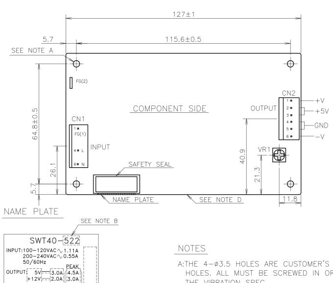
A:THE  $4-\phi 3.5$  HOLES ARE CUSTOMER'S CHASSIS MOUNTING HOLES. ALL MUST BE SCREWED IN ORDER TO CONFORM THE VIBRATION SPEC.
