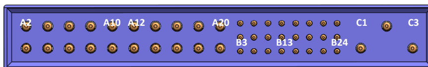
Figure 1-5: IN/OUTPUT CONNECTOR POSITRONIC P/N: PCIH47M400A1/AA
