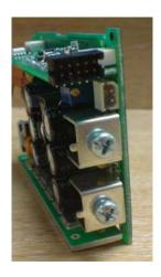
Figure 3. Module with required option board fitted.
