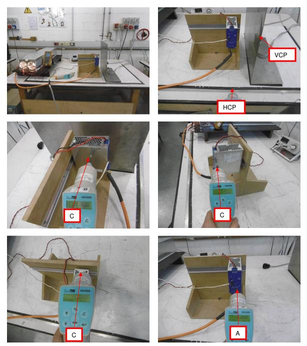
C = Contact Discharge / A = Air Discharge
