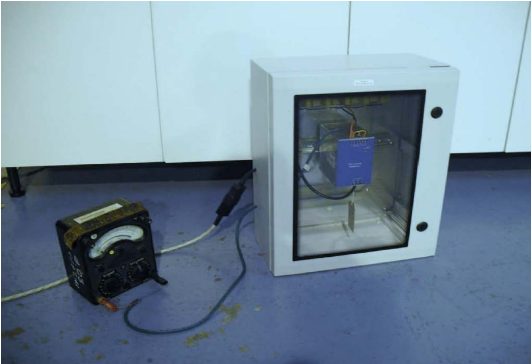
Figure 5 - Test Configuration, Radiated Emissions – In Cabinet
