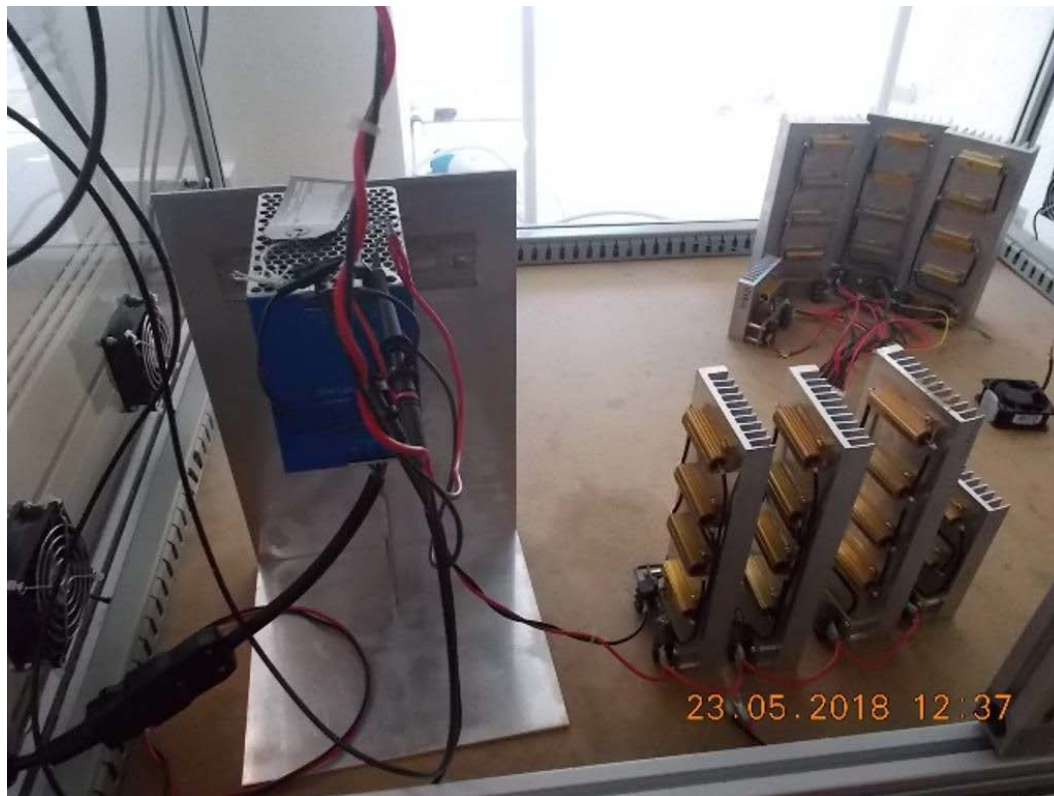
Figure 38 - Ring Wave, Test Setup, DRB480-48-1
