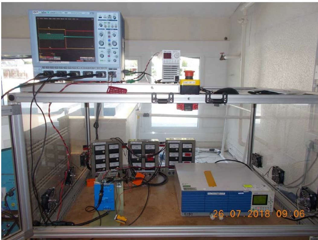
Figure 36 – Dips & Interruptions, Setup Photograph
