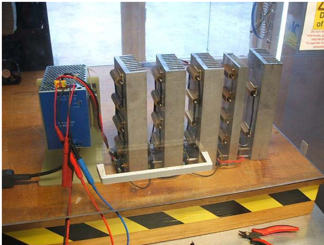
Figure 37 - Ring Wave, Test Setup, DRB480-24-1
