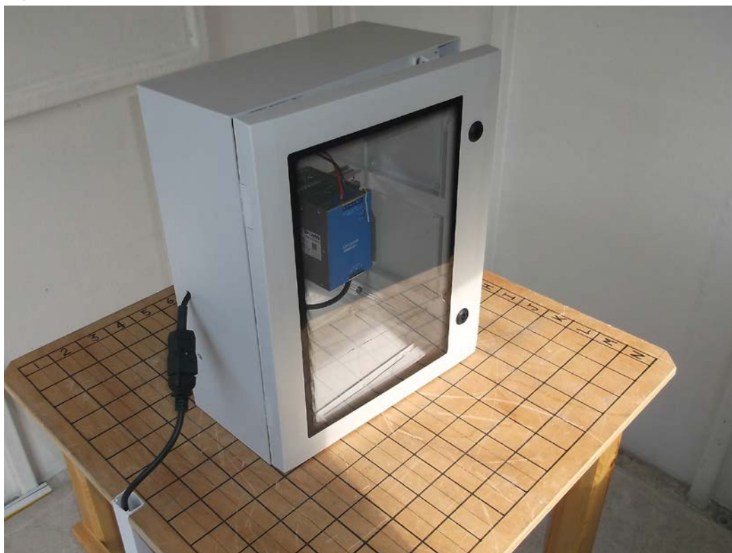
Figure 39 – Radiated Emissions Test Setup in Cabinet
