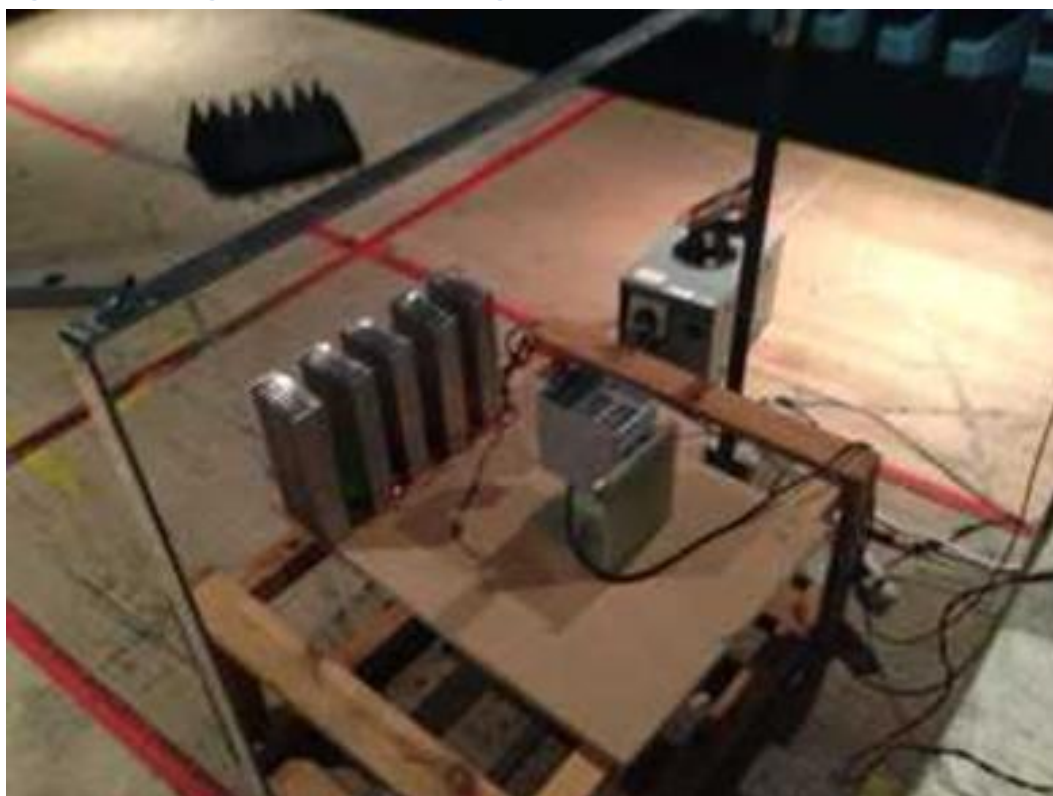
Figure 33 - PF Magnetic Field, Setup Photograph, X
