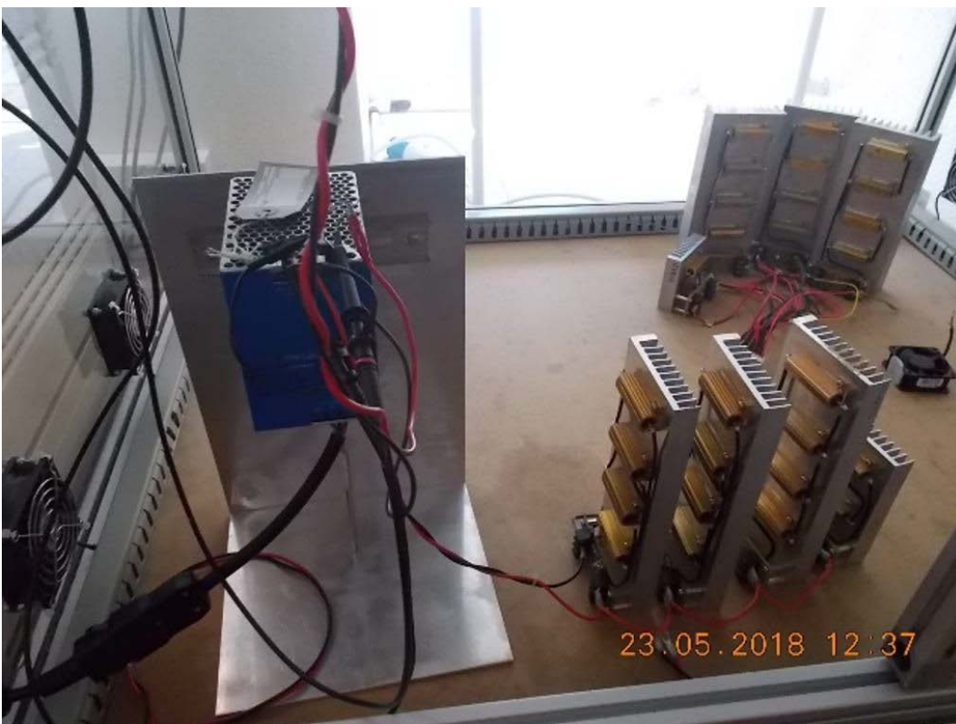
Figure 28 - Surge Immunity, Test Setup, DRB480-48-1
