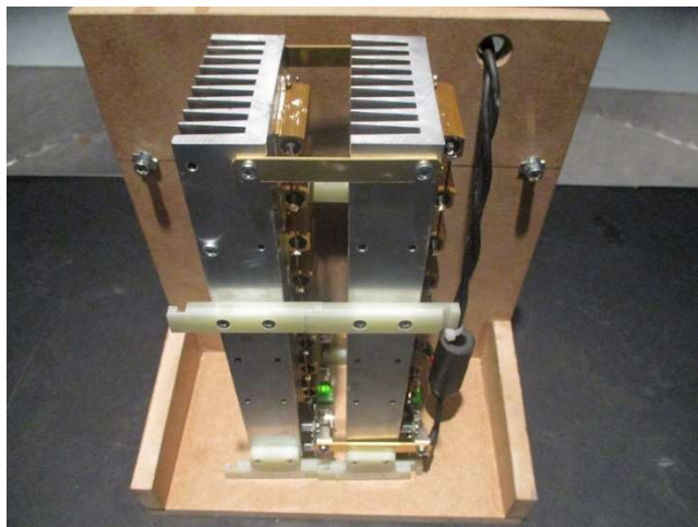
Auxiliary Equipment – Resistance load
