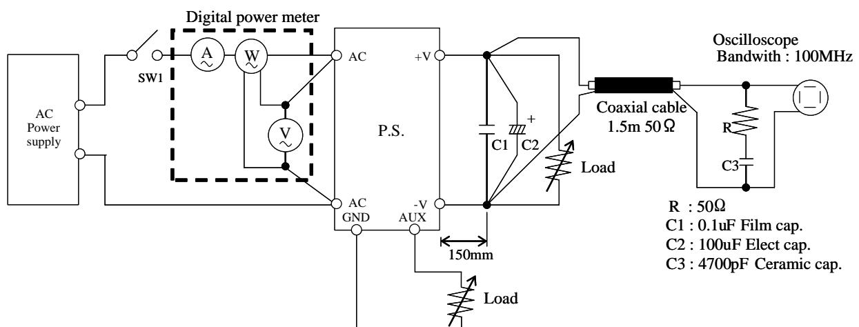
測定構成 Configuration used for determination
