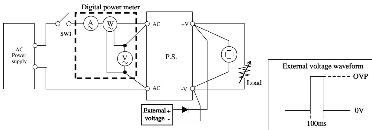
測定回路4 Circuit 4 used for determination
