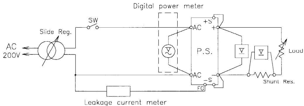
NOTE : Leakage current measured through a 1kohm resistor.
