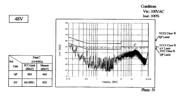
**Electro-Magnetic Interference characteristics**
