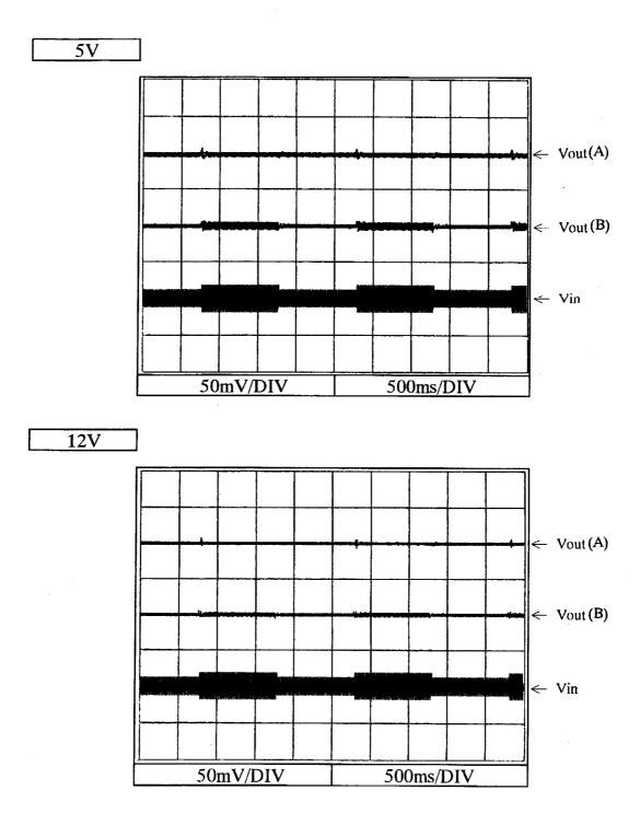
2.10 過渡応答(入力急変)特性 Dynamic line response characteristics
