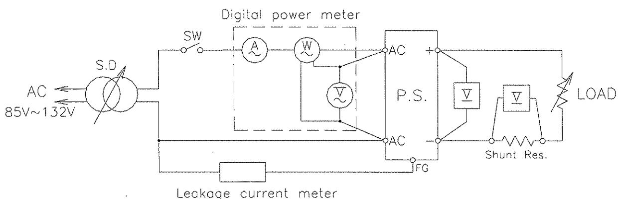
NOTE : Leakage current measured through a 1k ohm resistor.
