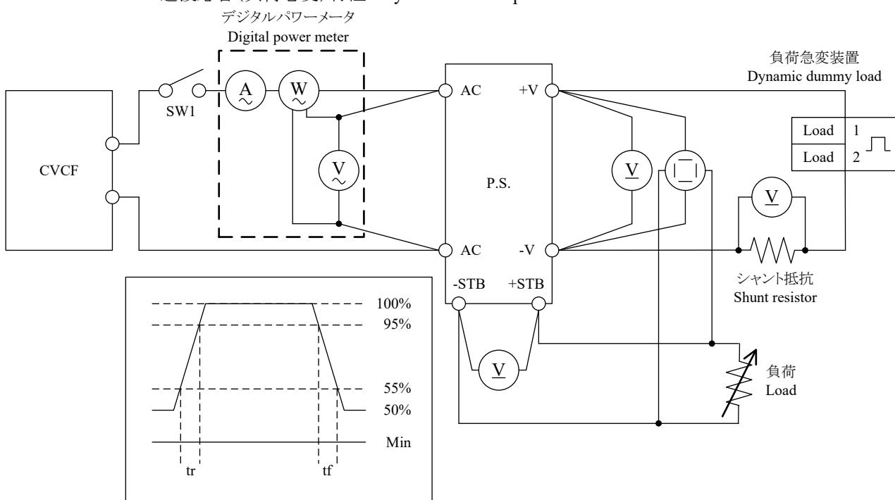
測定回路3 Circuit 3 used for determination
