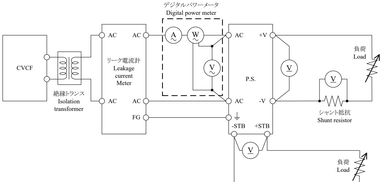
測定回路5 Circuit 5 used for determination
