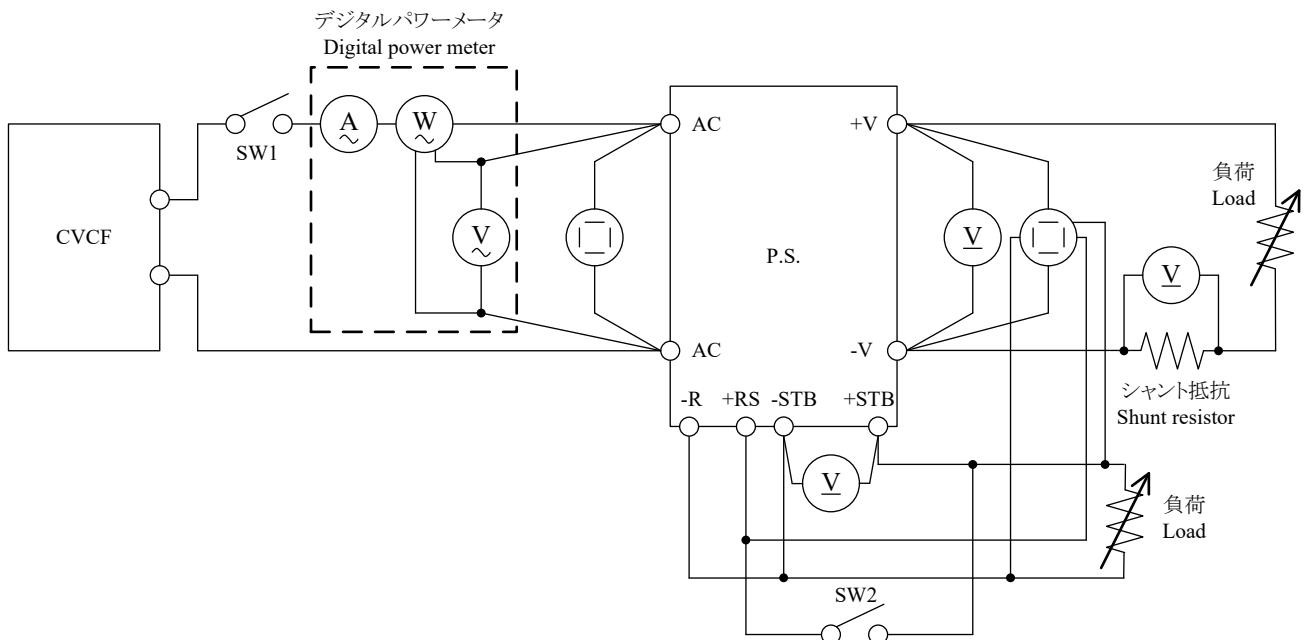
測定構成 Configuration used for determination
