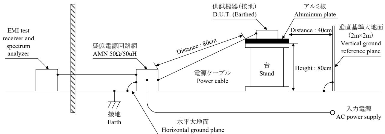
(b) 雑音電界強度(放射ノイズ) Radiated Emission
