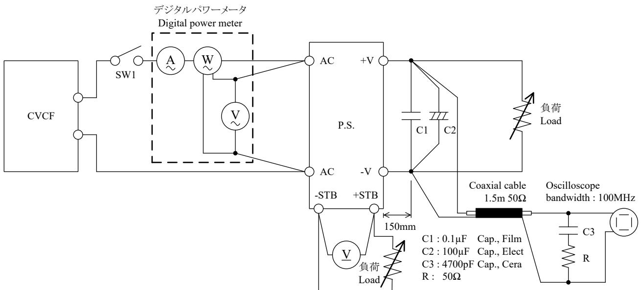
測定回路6 Circuit 6 used for determination
