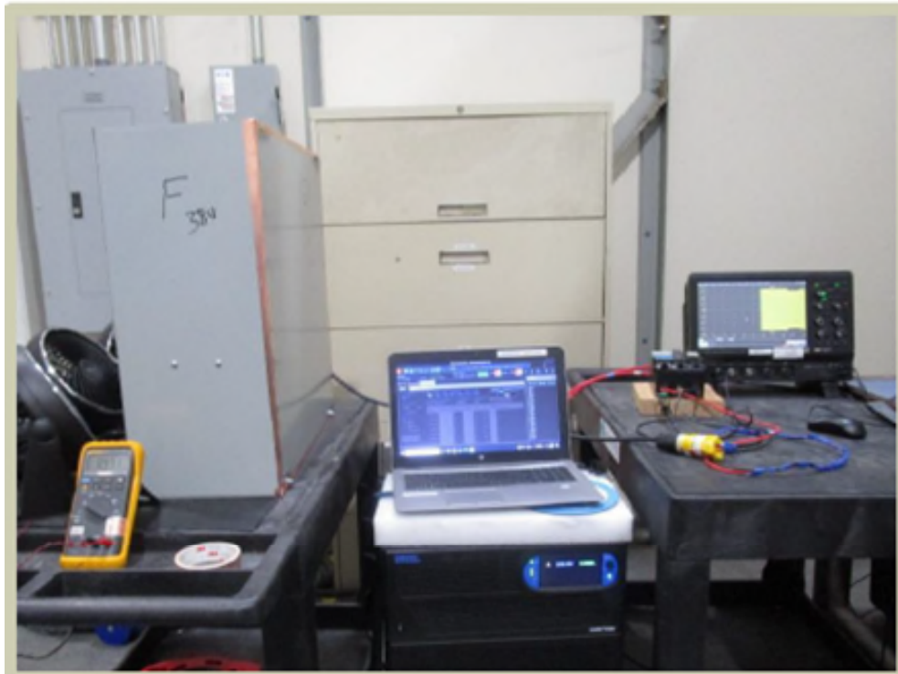
Test setup for Voltage Fluctuation Immunity.
