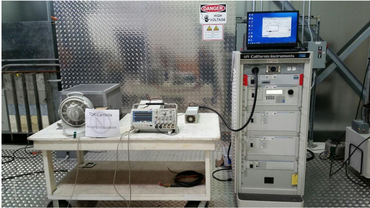
Voltage Dips and Interruptions Test Configuration Photograph
