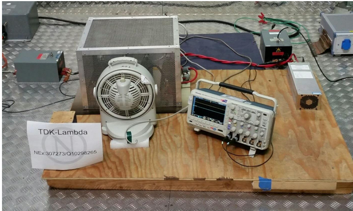
Continuous Conducted Disturbances Test Configuration Photograph
