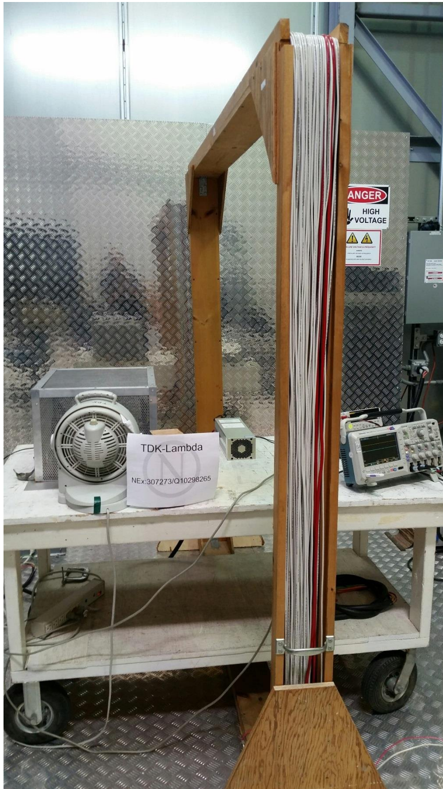
Power Frequency Magnetic Fields Test Configuration Photograph
