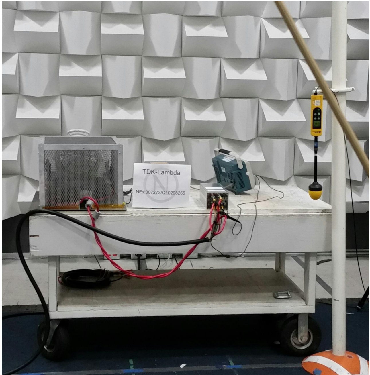
Continuous Radiated Disturbances Test Configuration Photograph
