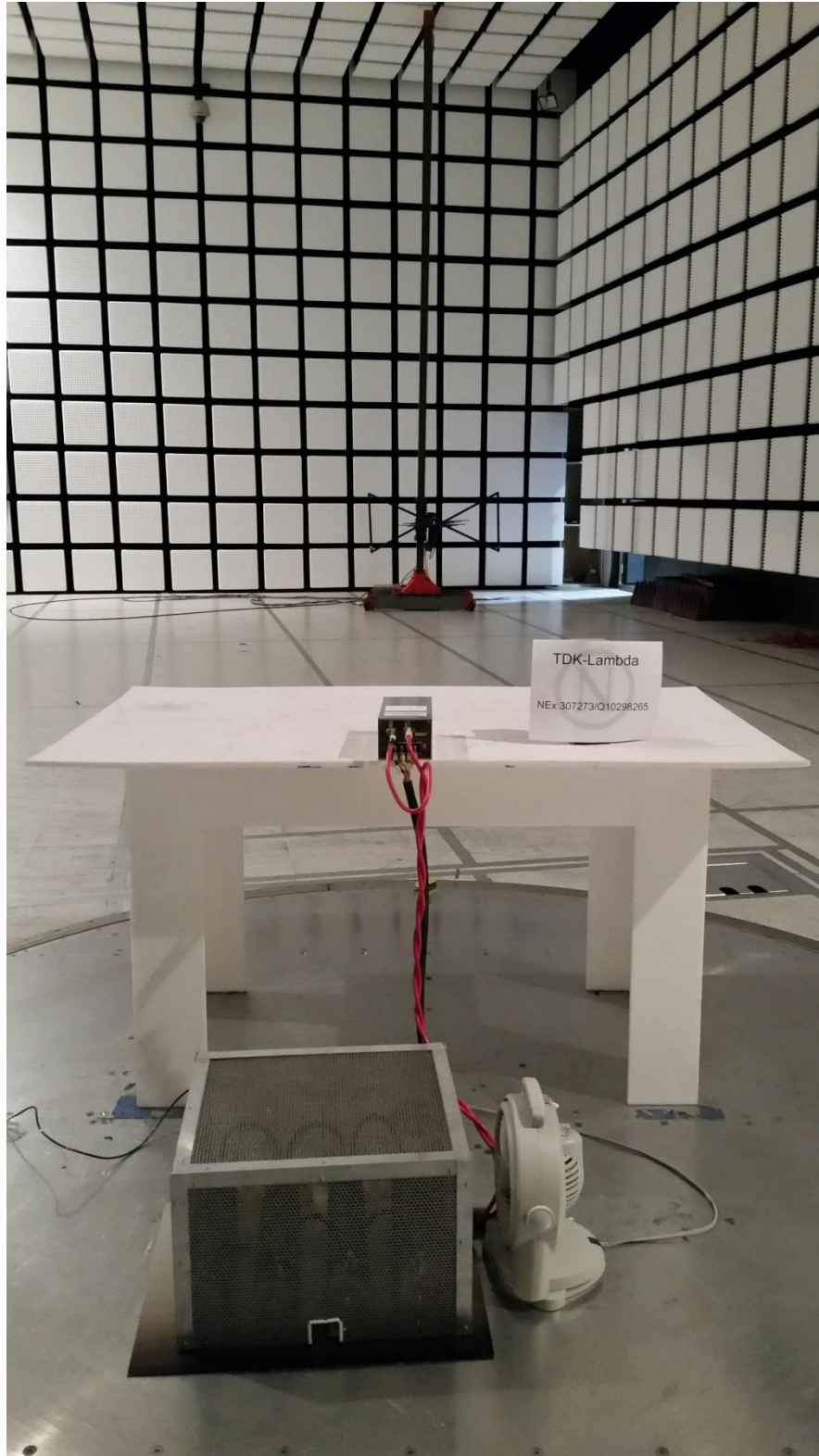
Radiated Emissions Test Configuration Photograph
