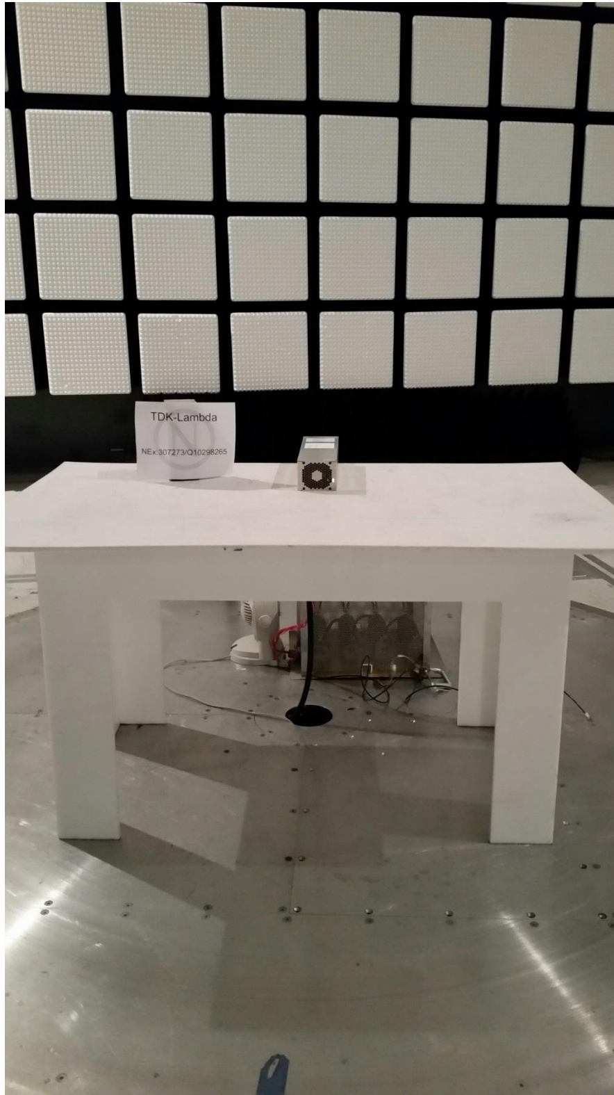
Radiated Emissions Test Configuration Photograph
