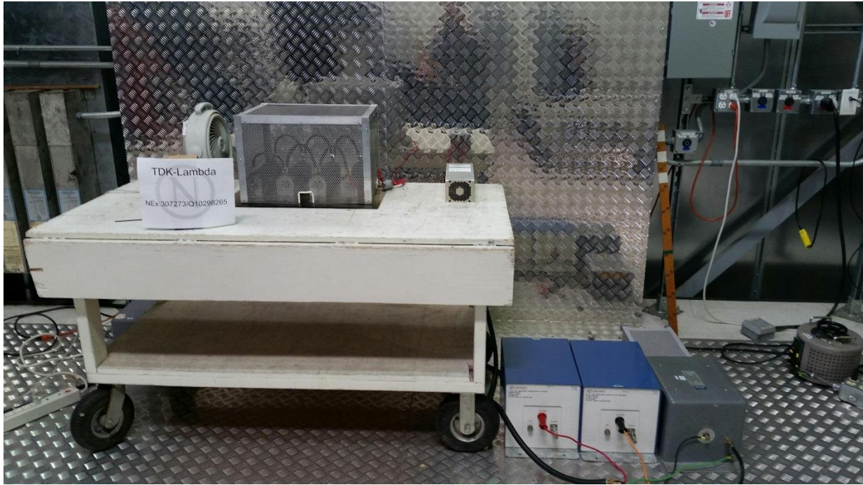
Conducted Emissions Test Configuration Photograph
