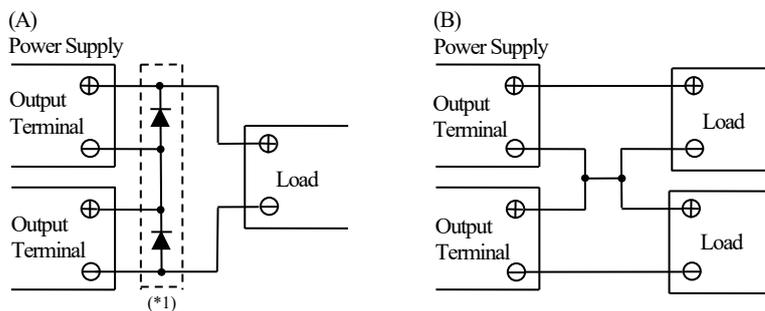
(\*1)Please select a bypass diode with maximum forward current rating more than output load current. And maximum reverse voltage must withstand each power supply output voltage.
