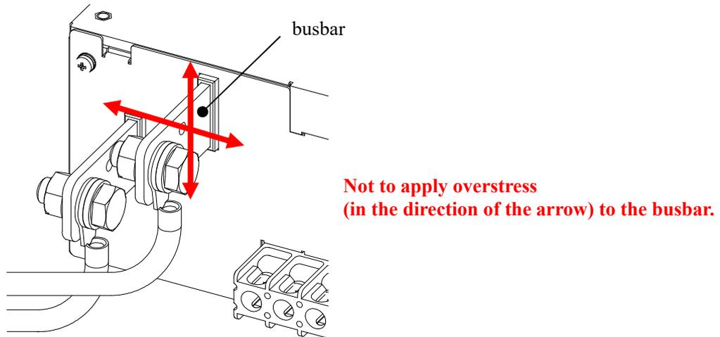
Example) Stabilize (supporting) the input/output terminals before tightening the screws.
