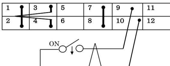
Connecting circuit with CN01 or CN02 connector
