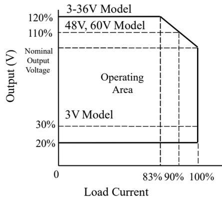
Note: Only as for the model of 48V, 60V output, the maximum output voltage is used up to 110% at 90% load current.
