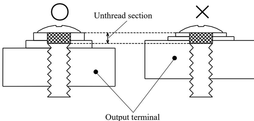
(9) Not to apply overstress to the busbar of the output terminal, as the output terminal part may be damaged.
