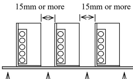
Provide punching, etc. to allow air to pass.
