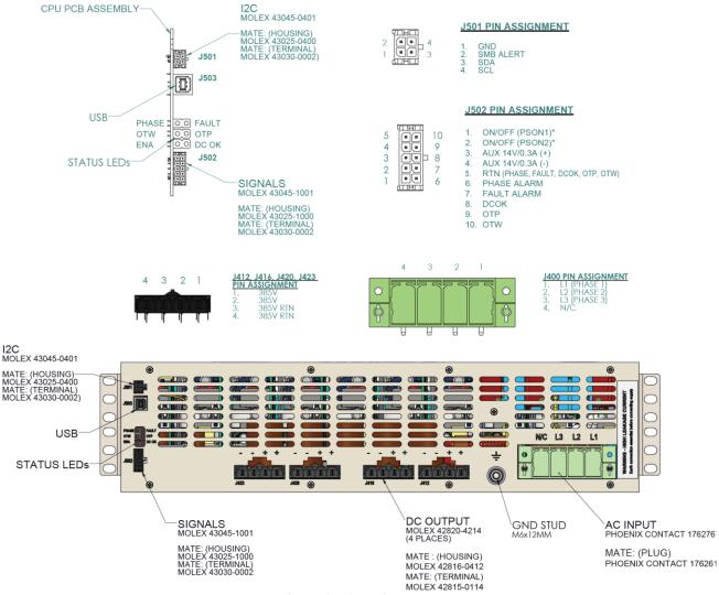
Figure 1: Pin assignments
