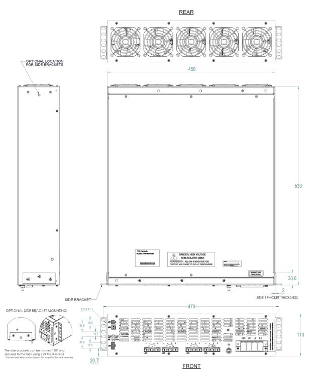
The unit weight is approximately 30 kg and should be installed onto a shelf or support bracket/rails. Secure in place using M6 or12/24 hardware into the two side brackets provided.
