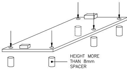
Please leave 4.5mm space from the unit surfaces and leave 4.5mm space from the sides of PCB. For the solder surface, 8mm space is necessary. If the space is not enough, the specification for insulation and withstand voltage will not be satisfied.
