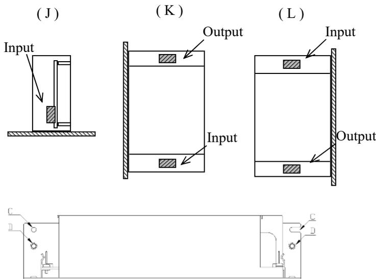
C: 1- $\Phi$ 4.5 holes and R2.25 slot hole by 2-M4 screws
