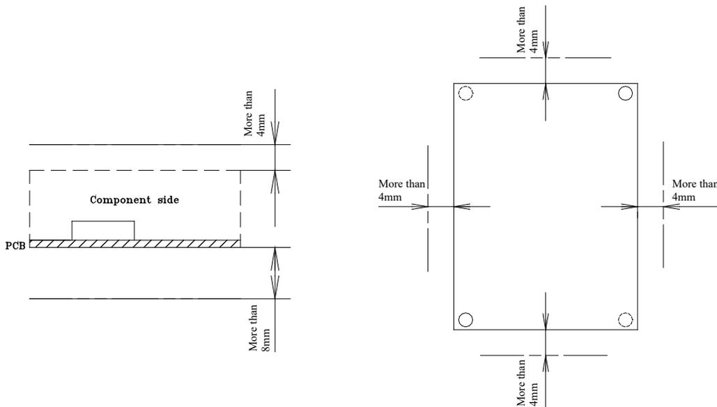
Keep 4mm space from the surfaces and sides of PCB. Especially, 8mm space is necessary from the solder surface. If the space is not enough, the specification of isolation and withstand will not be satisfied. Keep enough space in the power supply surroundings and the upper area of components for convection cooling.
