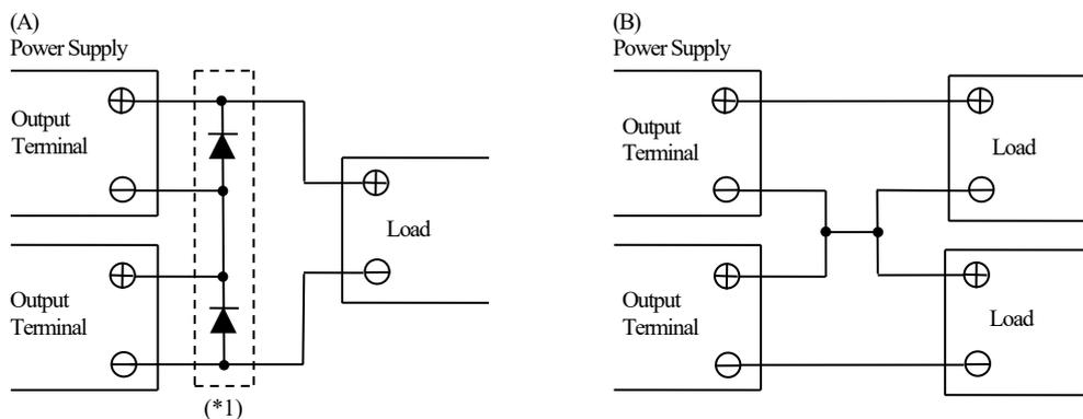
(\*1) Please select a bypass diode with maximum forward current rating more than output load current. And maximum reverse voltage must withstand each power supply output voltage.
