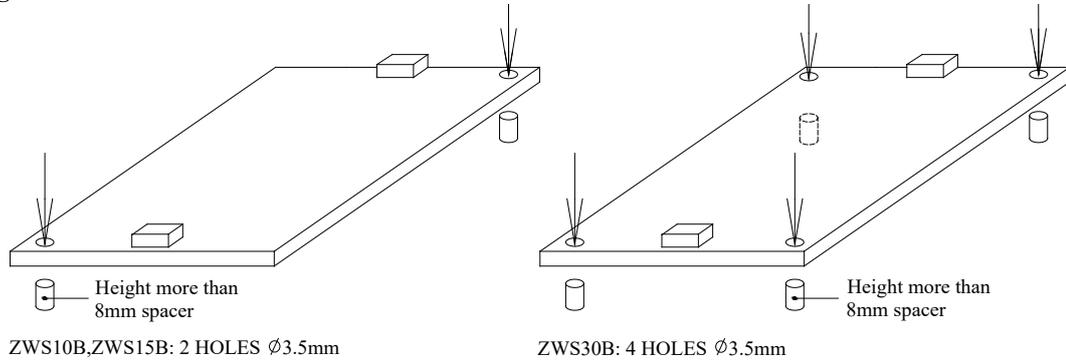
Allowable area by metal pieces is 8mm from each PCB corners. Refer to figure below.
