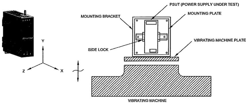
Fix the PSUT on the mounting rail with stopper on each corner.
