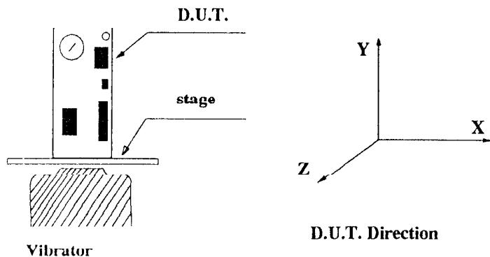
**Sweep frequency : 10 ~ 55Hz****Sweep time: 1min****Acceleration: const. (2G)****Direction: X, Y, Z.****Test time: 1H each****Result:**
