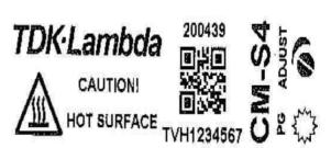
Note: The above markings are the minimum requirements required by the safety lab. For the final production samples, the additional markings which do not give rise to misunderstanding may be added.
