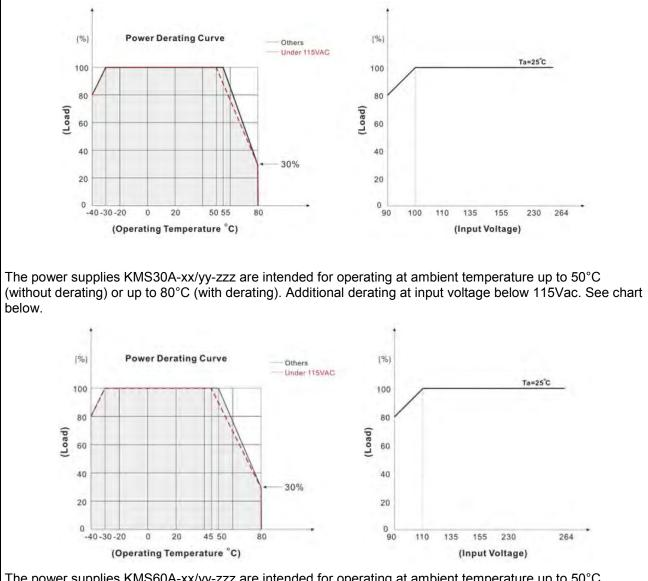
The power supplies KMS60A-xx/yy-zzz are intended for operating at ambient temperature up to 50°C (without derating) or up to 80°C (with derating):
