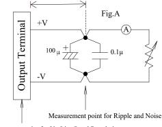
Measurement point for Vo Line/Load Regulation
