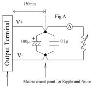
Measurement point for Vo Line/Load Regulation
