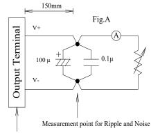
Measurement point for Vo Line/Load Regulation
