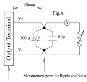
Measurement point for Vo Line/Load Regulation
