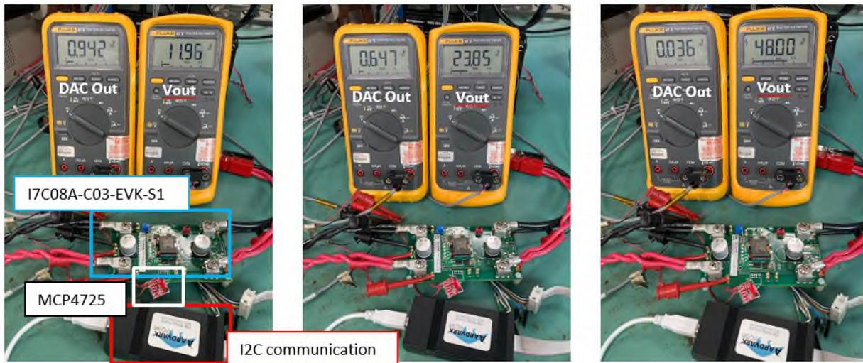
The output voltage equation determined previously was verified by experimental test result as shown in the photos.
