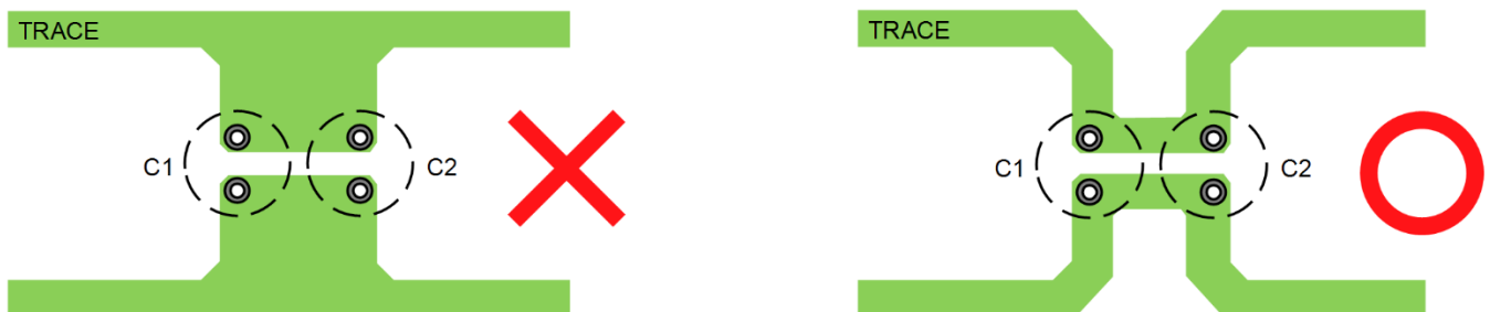
Fig. 3b: PCB Trace (incorrect PCB layout reduces ability to suppress Surge and EFT)
