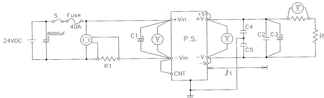
C1: 220uF Electrolytic Capacitor x 2para      C3: 48V-120uF Electrolytic Capacitor      R1: 0.01Ω
