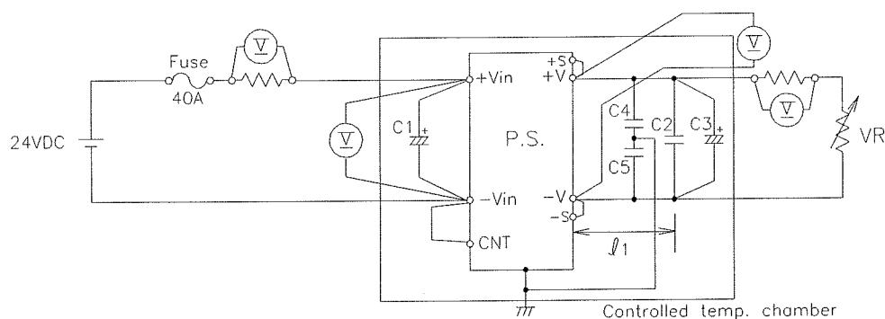
C1: 220uF Electrolytic Capacitor x 2para C3: 48V-120uF Electrolytic Capacitor l1: 50mm
