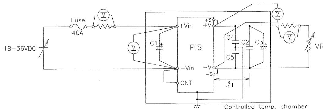
C1: 220uF Electrolytic Capacitor x 2para C3: 48V-120uF Electrolytic Capacitor l1: 50mm
