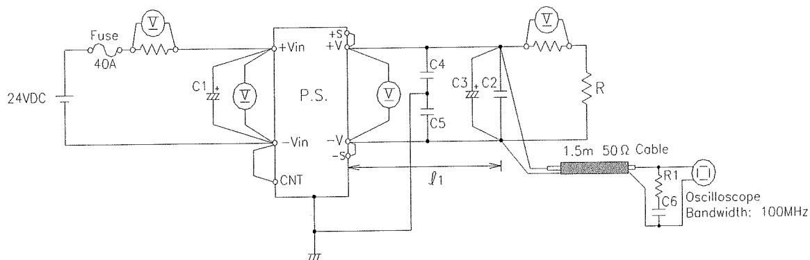
C1: 220uF Electrolytic Capacitor x 2para      C3: 48V-120uF Electrolytic Capacitor      C6: 4700pF Ceramic Capacitor
