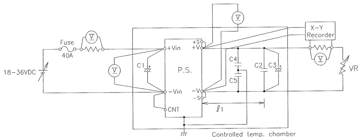
C1: 220uF Electrolytic Capacitor x 2para C3: 48V-120uF Electrolytic Capacitor l1: 50mm
