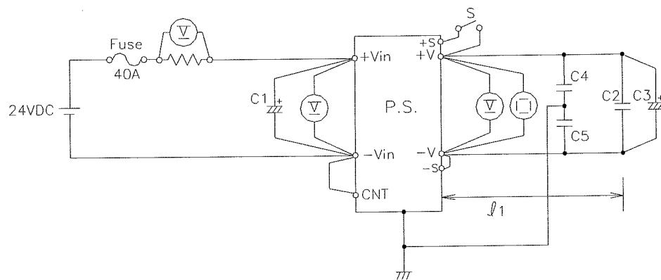
C1: 220uF Electrolytic Capacitor x 2para    C3: 48V-120uF Electrolytic Capacitor     $l_1$ : 50mm
