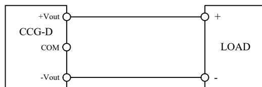
Fig.6-11 Connection when CCG-D single output is used
