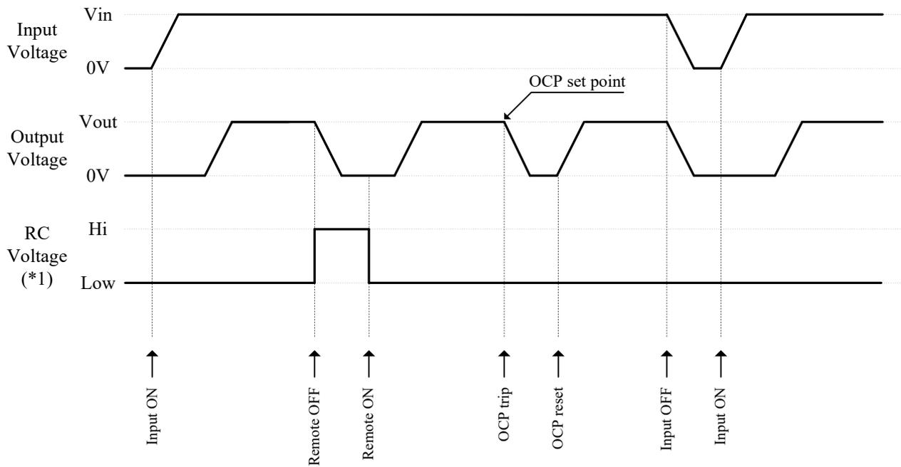
\*1 For example on above, RC Voltage shows Negative Logic control operation. For details on this function, please refer to Application Notes “6-7. Remote ON/OFF Control (RC terminal)” section.
