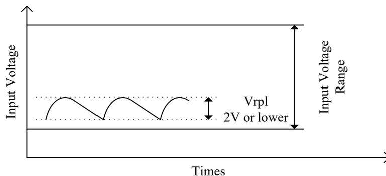
Fig.6-1 Input Ripple Voltage
