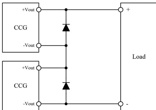
Fig.6-9 Series Operation for High Output Voltage
