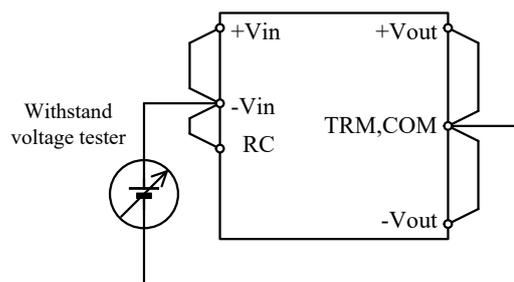
Fig.6-12 Withstand Voltage Test for Input - Output
