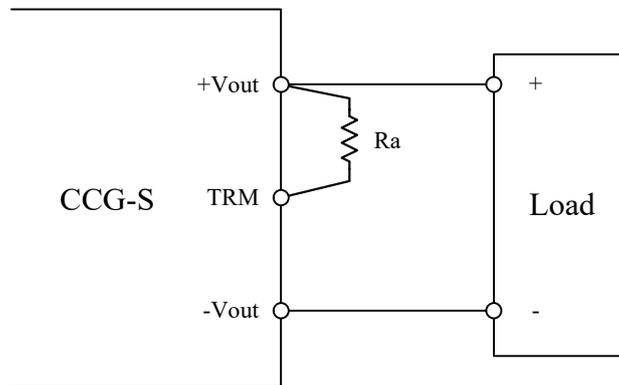
Fig.6-2 Basic Connection for Output Voltage Trim Down
