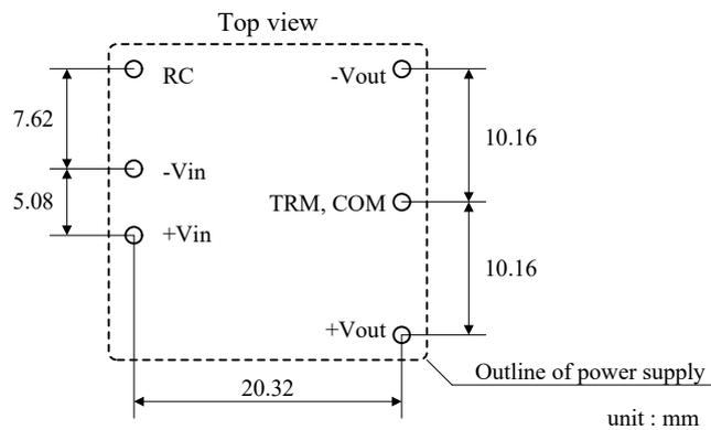
Fig.8-1 Dimension of Mounting Hole Position
