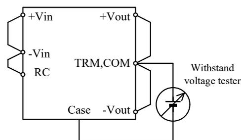
Fig.6-14 Withstand Voltage Test for Output - Case
