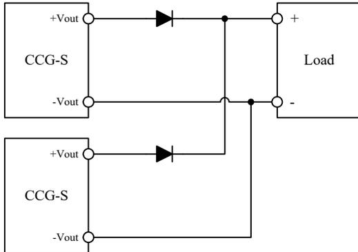
Fig.6-7 Redundant Operation Connection (CCG-S)
