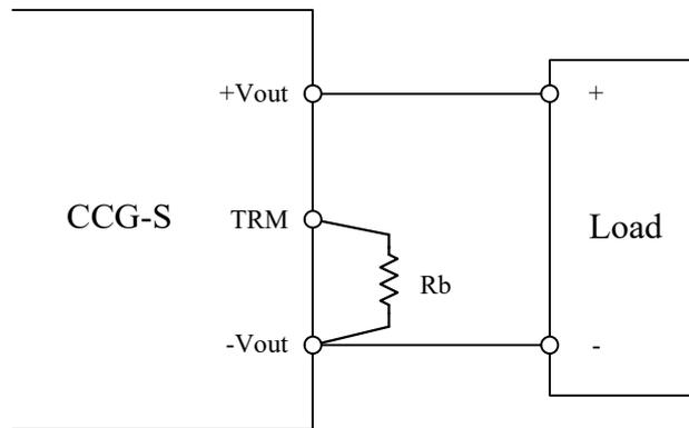
Fig.6-3 Basic Connection for Output Voltage Trim Up
