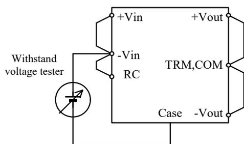
Fig.6-13 Withstand Voltage Test for Input - Case
