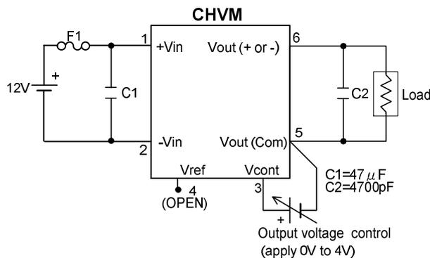
The CHVM series does not require any external parts, however when the impedance is high, for example: the distance between the power supply and converter is long, the input line is thin, or the input side has a filter then connecting a capacitor C1 to the input side is recommended. Place the capacitor as close as possible to the converter pin side, to lower the lead inductance.
