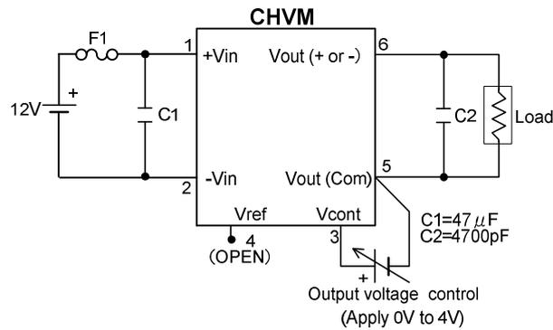
Warning 1: The ground line (2pin, 5pin) between the input/output, and the case are internally connected.
