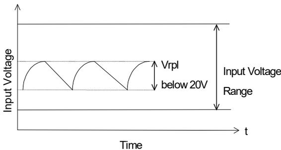
Fig.1-1 Ripple Voltage
