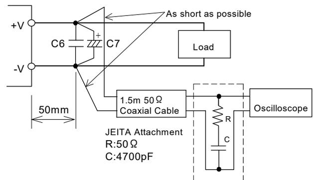
**Fig.3-1 Measurement of Maximum Output Ripple & Noise**
