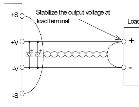
Fig.9-1 Remote Sensing at Use
