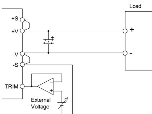
**Fig.2-3 Output Voltage Adjustment by applying external voltage**
