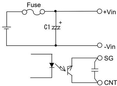
Fig.10-1 CNT,SG terminal connection
