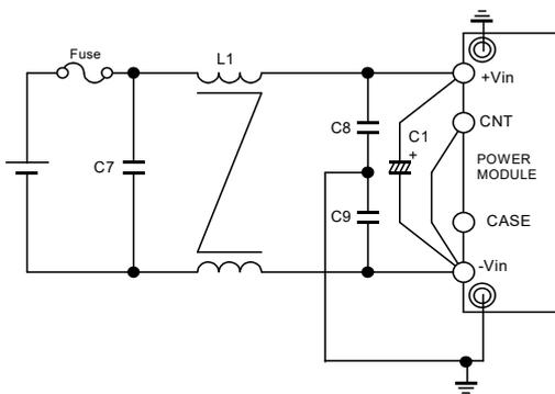
Fig.1-7 Recommended input filter as EMI countermeasure (2)
