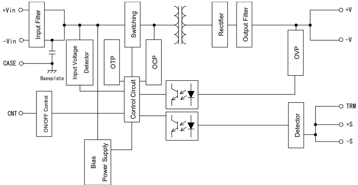
Switching Frequency (fixed) : 370kHz (typ.)
