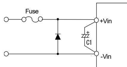
**Fig.1-5 Protection for Reversed Connection of Input**
