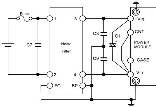
Fig.1-6 Recommended input filter as EMI countermeasure (1)
