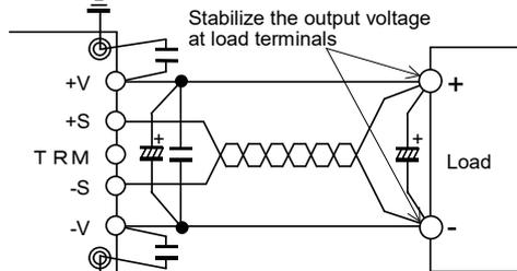
**Fig.9-1 Remote Sensing is in Use**
