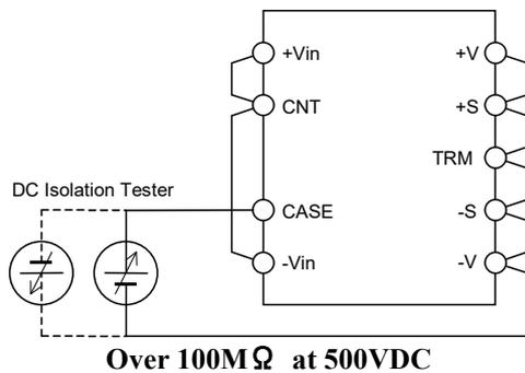
**Fig.20-1 Isolation Test**
