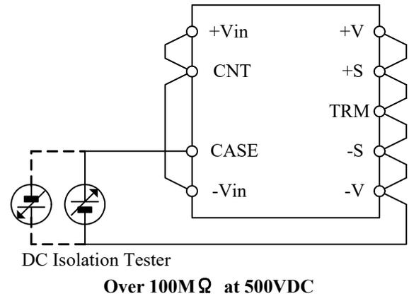
**Fig.20-1 Isolation Test**
