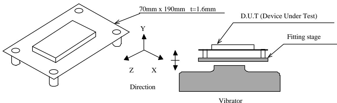
Put the D.U.T. on the universal circuit board (soldering Input Output signal terminals and fixing by four M3-tapped-holes) and fit it on the fitting-stage.
