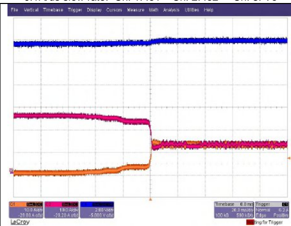
Start-up with back-biasing: Vin=48V, Io=25A Ch. 1: Io1 Ch. 2: Io2 Ch. 3: Vo
