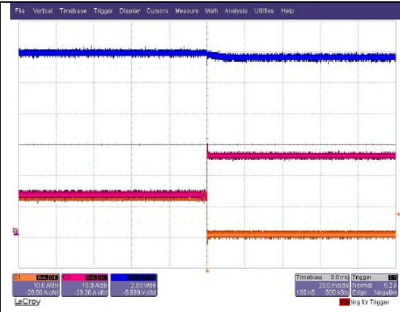
Shut-down when running Io=50A load (200% Load) Ch. 1: Io1 Ch. 2: Io2 Ch. 3: Vo
