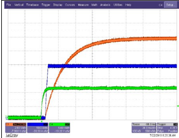
Start-up from on/off Switch at 48V input and Full Load. Ch. 1: Vo Ch. 3: Io Ch. 4: ON/OFF
