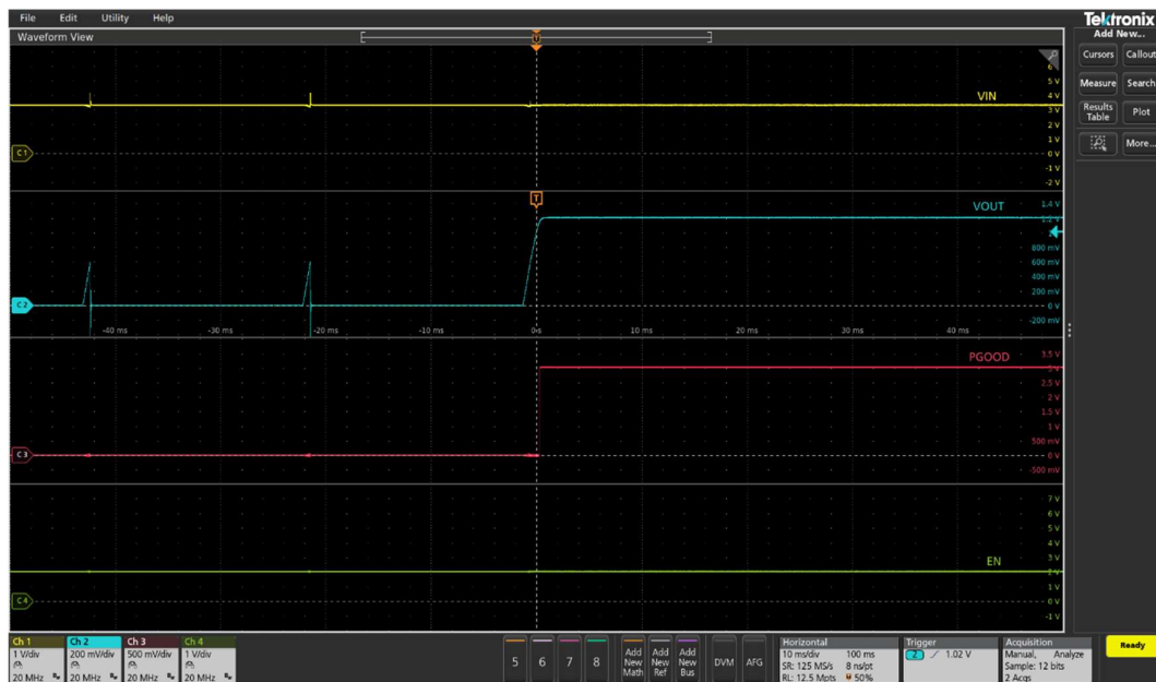
Figure 14 Recovery from OCP (Ch1: V_{IN} , Ch2: V_{OUT} , Ch3: PGOOD, Ch4: EN)
