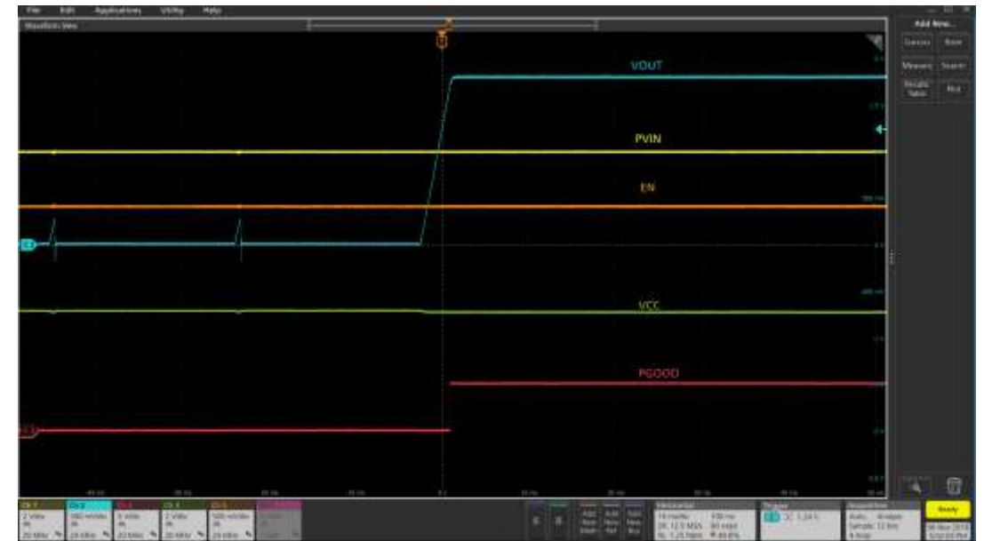
Over Current Protection and Auto Recover to 6A Ch 1: PVin Ch2: Vo Ch3: PGood Ch4: Vcc, Ch 5: En
