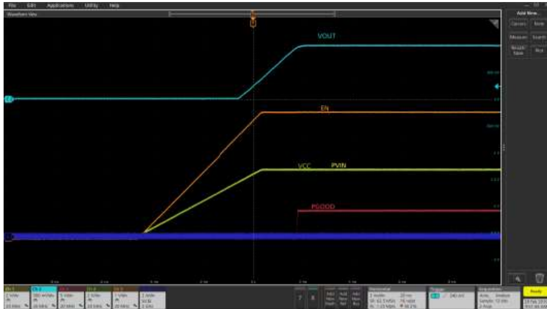
Start Up @ 0A Ch1:Vin Ch2:Vo Ch3:PGood Ch4:Vcc Ch5:En Ch6:Iout
