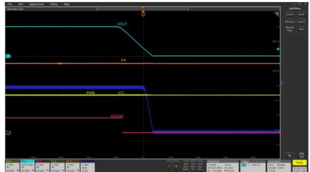
Soft turn off @ 6A Ch1:Vin Ch2:Vo Ch3:PGood Ch4:Vcc Ch5:En Ch6:Iout
