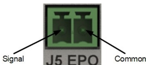
Figure 8-5: Emergency Power OFF (EPO) Connector
