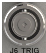
Figure 8-6: Trigger Out Connector
